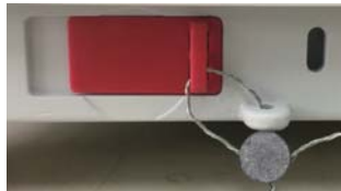
Locked with Wire Seal
